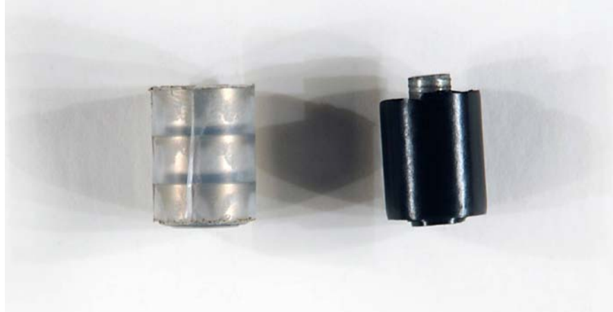
Figure 4: The button batteries on the left have been insulated by wrapping them in a single layer of transparent tape. The picture on the right shows a replacement for the button batteries if the pointer will be attached to an external power supply. It is a piece of metal rod (the rod needs to be conducting) wrapped with electrical tape so that it fits snugly into the pointer.
