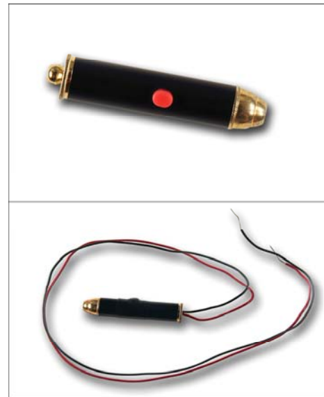
Figure 2: Bullet-type laser pointer before and after modification. Note the Knob on the left end was cut off with a hacksaw before drilling a hole in the end cap.
